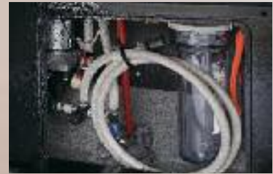
WINTERIZING TUBE Easy access for quick maintenance includes bypass valve.
